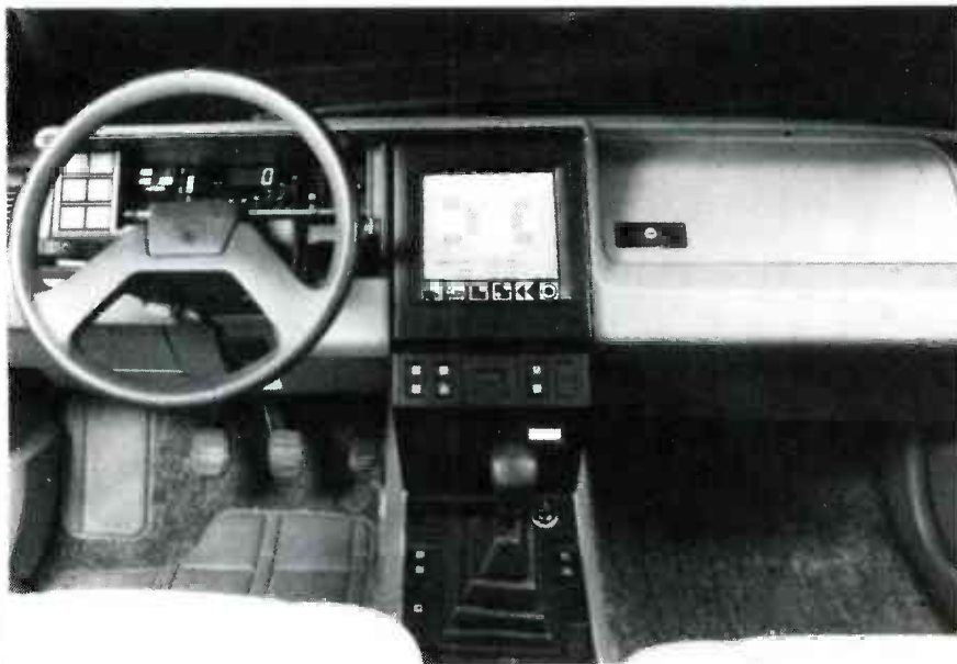
VOTAN-VOICE RECOGNITION TECHNOLOGY enables the Renault to obey "its master's voice." The system allows the driver of the demonstration car to control non-critical accessories, such as windshield wipers, windows, radio, heater, and air conditioner.
