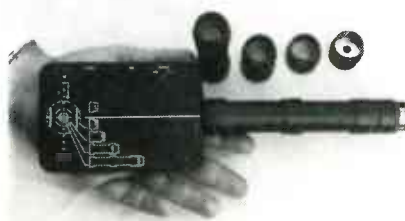
FIG. 14—THE MICROSCANNER can measure temperature from a distance by using special lenses.
