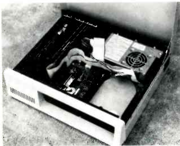
FIG. 7—THE DISK-DRIVE CABLES should be mounted so that they are neat and out of the way of any moving parts.
