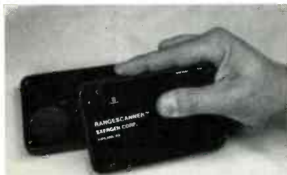
FIG. 13—THE ULTRASONIC RANGESCANNER measures distance and uses a Polapulse battery for power.
