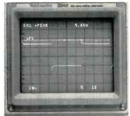
FIG. 6—MEASUREMENT CURSORS are positioned by the oscilloscope automatically. They give visual confirmation that the appropriate region of the waveform is being measured.
