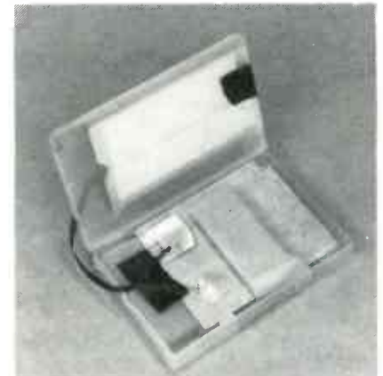
FIG. 18—A USED P100 BATTERY can be mounted in a discarded audio-cassette box.
