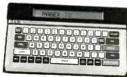
FIG. 16—THE TC200 is a portable telecomputer that provides 8K of RAM and a built-in modem. It's powered by a P500.
